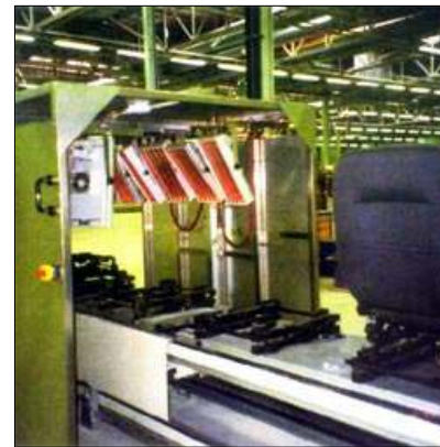
Heating of mouldings and of the zones where they have to be mounted
