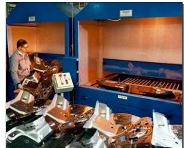
Treatment of soundproofing panels, before their installation
