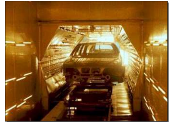
Drying of varnish and primer
