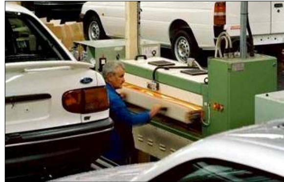
Heating of mouldings and of the zones where they have to be mounted
